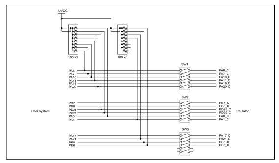
Figure 3 Circuit for Masking Signals
